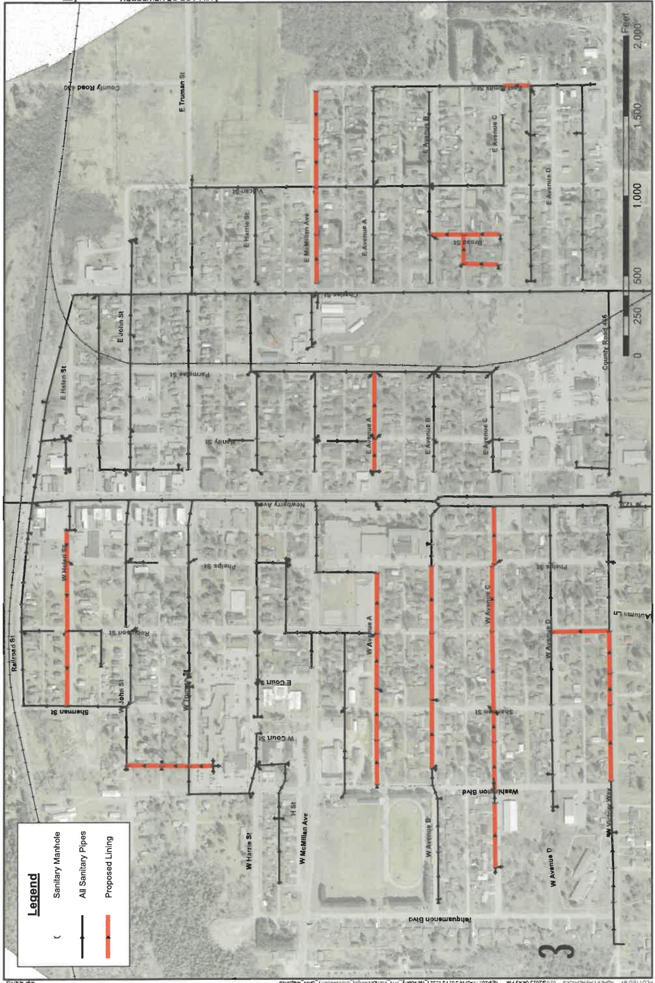
FIGURE 1. PROPOSED WASTEWATER LINING AREAS
